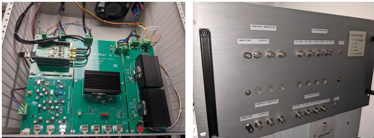
FIG. 3: PHOTOS OF THE COMBINED ANALOG AC+DC POWER SUPPLY DESIGNED AND TESTED AT UCL. LEFT: THE ACTUALLY PRODUCED ELECTRONIC CIRCUITS. RIGHT: THE INTERFACE FOR THE EXPERIMENTS.
