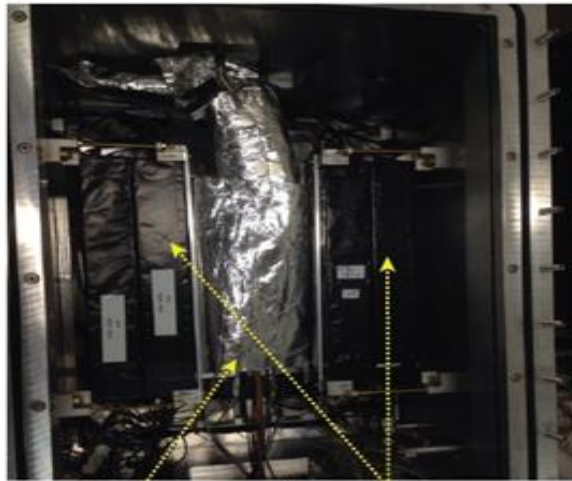
heat insulator wrapped around the SDDs side scintillators
