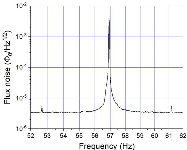
FIG. 2: Typical power spectrum of the  $z$ -mode over 12 hours, acquired at a pressure  $P = 5.6 \times 10^{-5}$  mbar. The two small satellites correspond to a nonlinear mixing with an horizontal mode at 4.3 Hz
